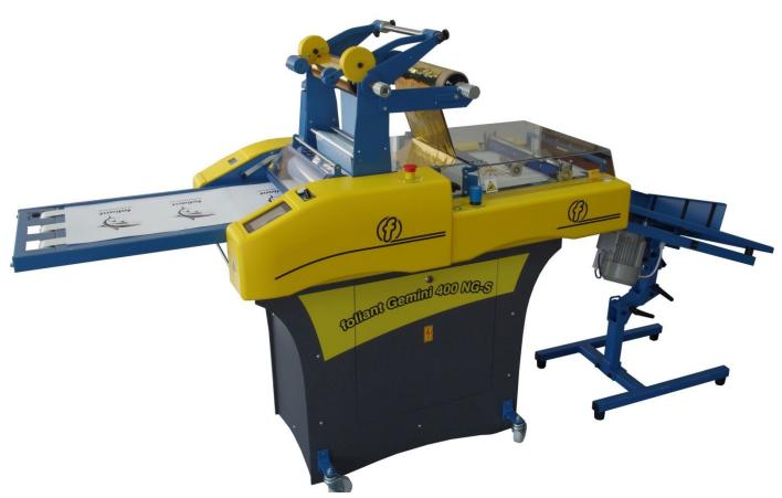
The machine's main feature is a pneumatic pressure system in a heavy duty mechanism enabling to achieve a very high working pressure, one single phase 220 – 240 V supply cable, a small integrated compressor inside the machine frame (i.e. no external source of pressured air is required), a nice design and an easy machine operation.
